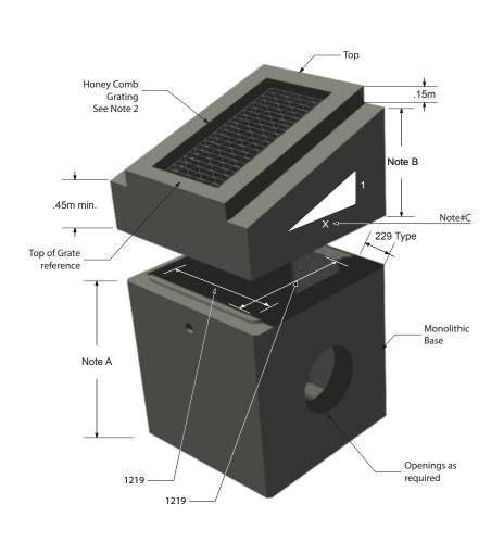
A- Monolithic Base heights as follows: .61m - 1.53m @ .15m increments B- Riser Top Section heights as follows: .45m - 1.22m @ .15m increments
