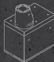
Ditch Inlet Flat Cap (mass - 742 kg + 1133 kg/m)
