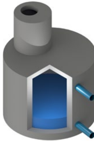
ROUND SWRS - MAINTENANCE HOLES
