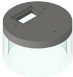
Ditch Inlet Type A
