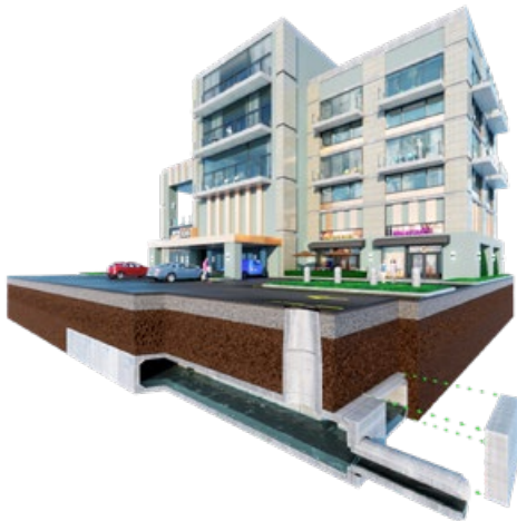
TWIN BOX CULVERT SWRS
