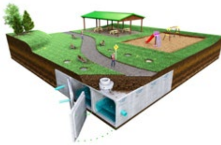
TRIPLE BOX CULVERT SWRS
